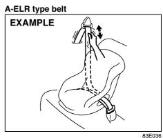
Make sure that the retractor has converted to the ALR mode by trying to pull webbing out of the retractor. If the retractor is in the ALR mode, the belt will be locked.
